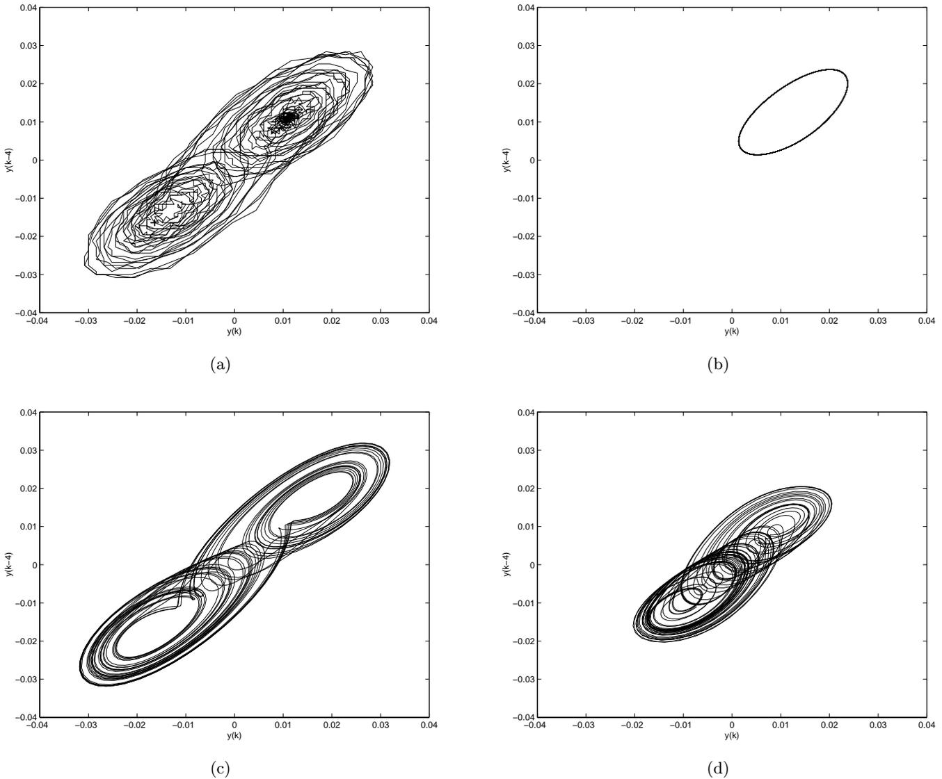
Fig. 3. Bidimensional projection of reconstructed attractors of Chua's circuit. (a) Identification data attractor. Note the low signal to noise ratio due to digitalization, (b) attractor of identified model (13), (c) attractor obtained for  $\tilde{a}_1 = 1.4902$ . (d) Model obtained through variation in  $\tilde{a}_3 = -2.0263 \times 10^3$ .
