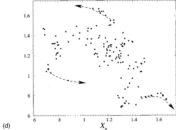
FIG. 4. First-return maps to the Poincaré section for four different values of the discharge current  $I$ . The three unstable periodic points are drawn by hand in order to clarify the relative organization between the torus and the unstable periodic orbit. The heteroclinic connections are represented by dashed lines. 130 points are recorded in the Poincaré section.
