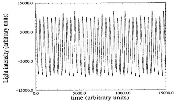
FIG. 2. Time series of the light intensity recorded near the cathode by using a photodiode ( $I=30.4$  mA).
