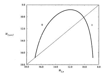
FIG. 5. First-return map of the image system of the simplest equivariant chaotic system just before the attractor merging crisis ( $\alpha = 2.027717$ ). A similar map may be obtained using the  $u_3$  variable.
