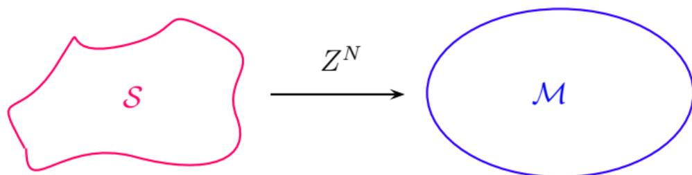
**Figure:** Simplified schematic diagram for *black-box identification*, where  $S$  represents the system that should be approximated by a model  $M$  which is built from a set of measured data  $Z^N$  of length  $N$ .
