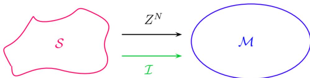
**Figure:** Simplified schematic diagram for *grey-box identification*, where  $\mathcal{S}$  represents the system that should be approximated by a model  $\mathcal{M}$  which is built from a set of measured data  $Z^N$  of length  $N$  and auxiliary information  $\mathcal{I}$ .
